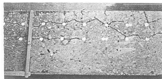
Photo 1 Internal Cracks Spanning Heated Reinforcing Bars, Observed After Cutting with a Diamond Saw.
